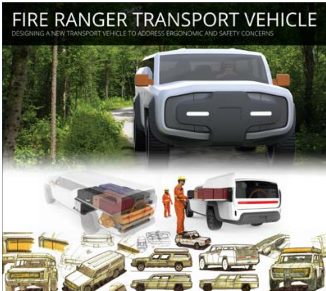
Industrial Design student Kyle Lunau created a design for a Fire Ranger Transport Vehicle that addresses issues with the existing trucks used by forest fire rangers in Northern Ontario. It includes a pull-out cargo tray system to solve ergonomic issues, as well as significant considerations for visibility and overall safety.
