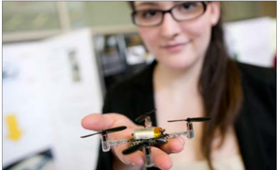
Electrical Engineering student Melissa Stapleton holds a Crazyflie nano-quadcopter. Melissa was part of a team of capstone project students that used the Crazyflie, a purchased product, as an open-source platform for the development of avionic equipment. Her team looked specifically at control systems, sensors, communications, power systems and swarm intelligence on micro-UAV platforms.
